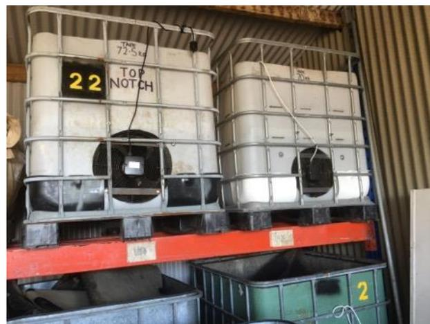
For hoppers they have developed a system that both carries and dries the nuts, made from a standard agricultural cube container with the top cut out and a bottom trapdoor-controlled chute and a fan that blows air through the nuts. These affordable hoppers can take half a tonne of nuts.
